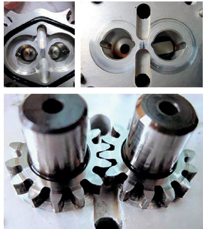
The main cause of component failure of a hydraulic circuit is due to dirt in the oil, produced by the deterioration of the same, high working temperatures, a lack of maintenance.
