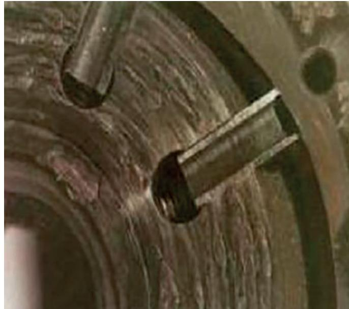
Premature wear on body and gears of an external gear pump.
